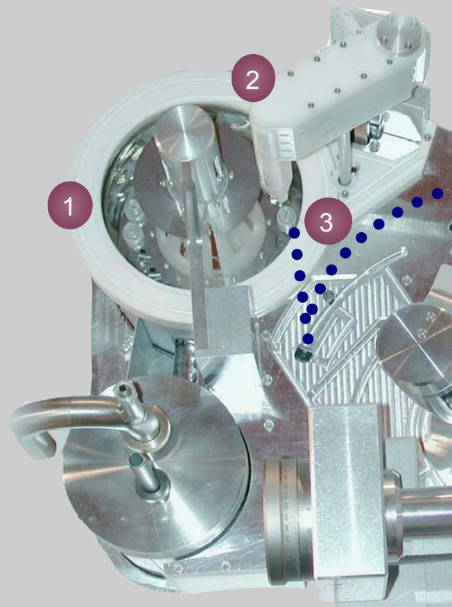
⑥ The vial server pushes the vial up towards the magnetic base of the goniometer head.
