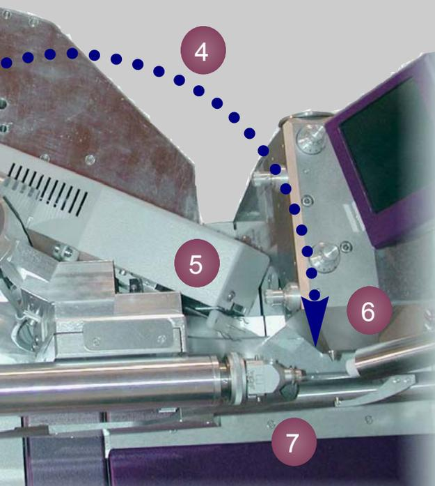
⑤ The vial server pushes the vial close to the collimator and into the cold stream.
