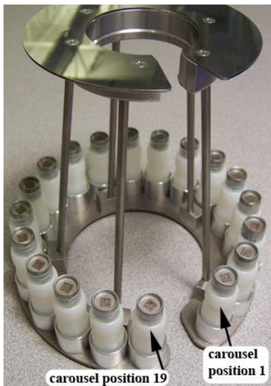
Figure 44 - MarCSC carousel. Positions 1 and 19 are indicated.
