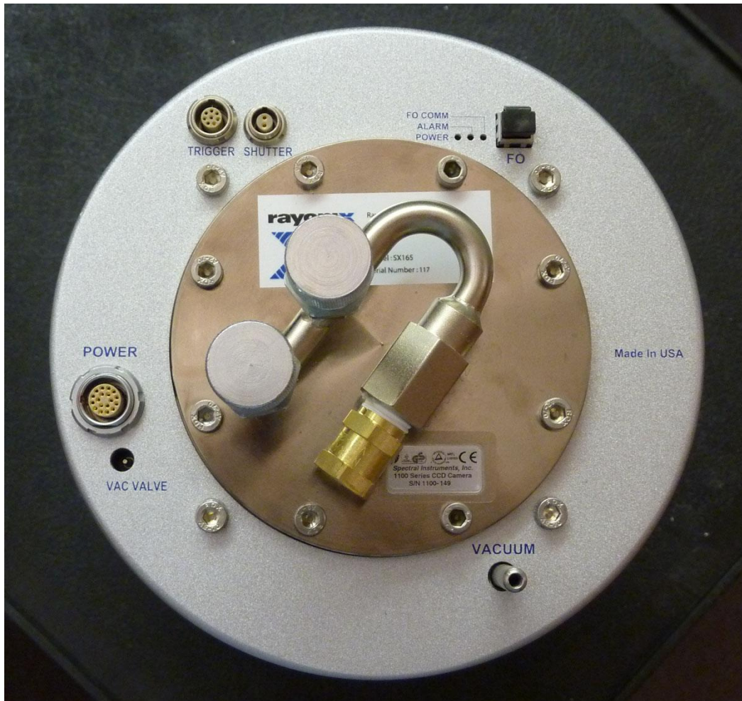
Figure 35 – SX Series detector head, rear view
