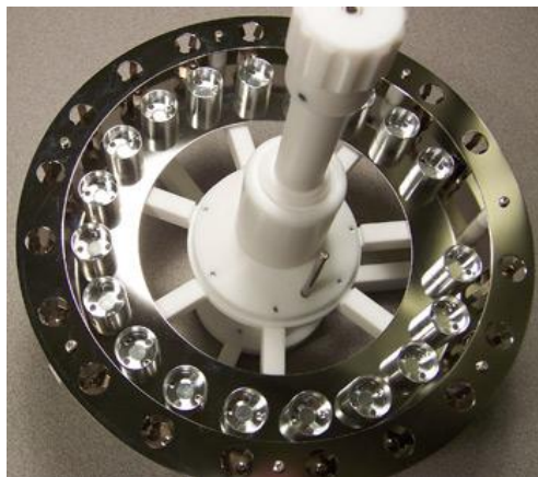
Figure 45 - Sample Transfer Station
