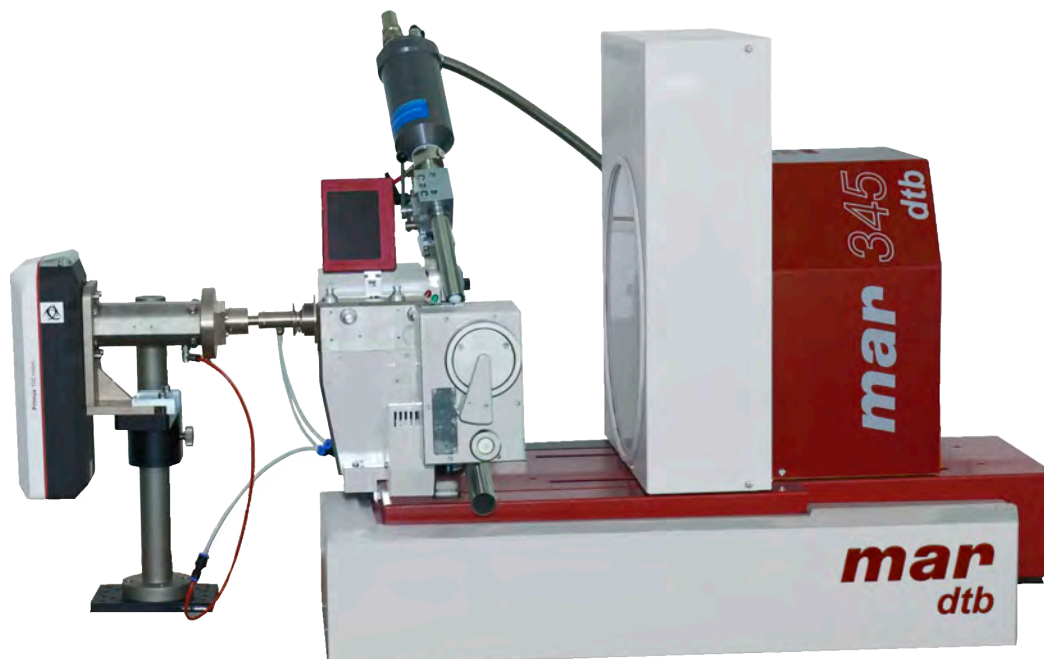
mar \mu X 3G : Primux/ASTIX++ with mar345 detector and mar dtb goniostat
