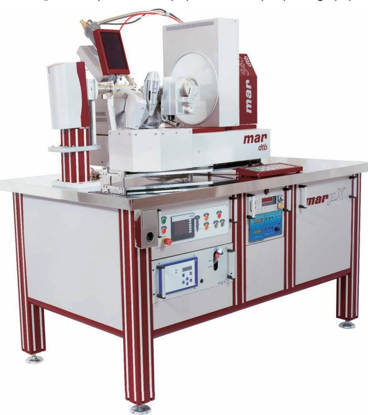
mar μX is a complete turn-key system for X-ray crystallography of single crystals. mar μX consists of a micro-beam X-ray generator operating at 30 Watts, producing a 20 μm microfocus spot. It is equipped with a modern multi-layer optic producing
