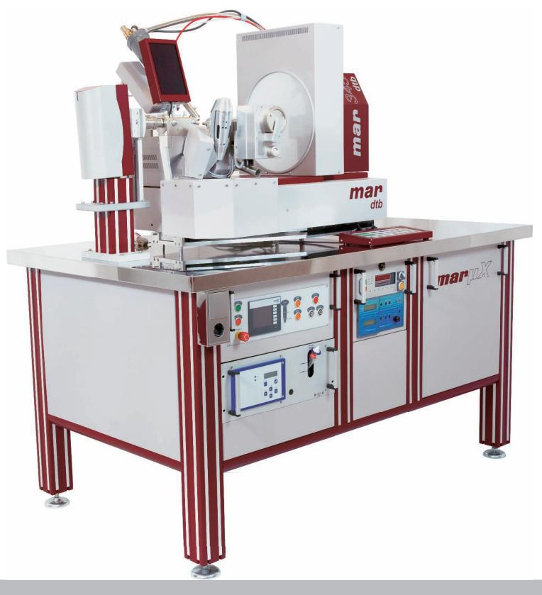
**mar**  $\mu$  X is a complete turn-key system for X-ray crystallography of single crystals. **mar**  $\mu$  X consists of a micro-beam X-ray generator operating at 30 Watts, producing a 20  $\mu$ m microfocus spot. It is equipped with a modern multi-layer optic producing
