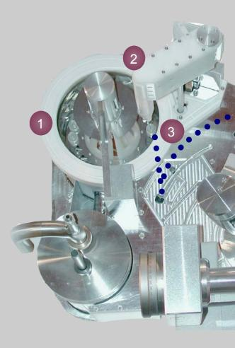
**6** The vial server pushes the vial up towards the magnetic base of the goniometer head.
